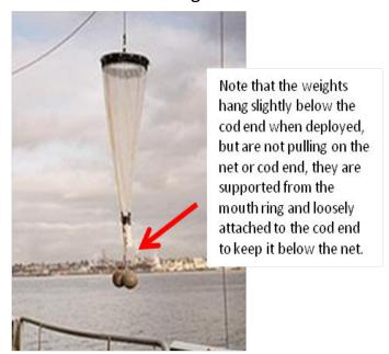
that the line to the cod end isn't so short that it will stretch the net toward the weight when deployed – that could rip the net. **The net and cod end should never feel the weight.** Attach weights to the O-ring before deployment. [Weighted cod ends are available, but aren't heavy enough to sink the net vertically except when it's very calm.]
