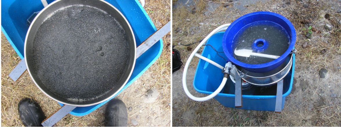
Figure 3. A sieve (left) and winnowing setup (right) used for initial processing of samples. The winnowing setup separates eggs from sand as much as possible, by creating a gentle vortex and using the eggs' natural buoyancy to capture them from the water's surface. Photo credit Tim Cochnauer.
