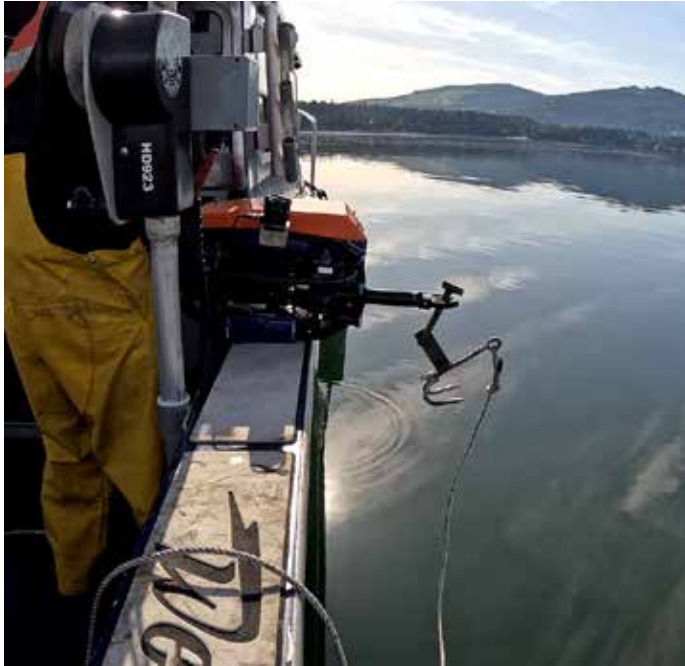
Figure 1. ROV with gripper, holding large fish hook and separate line aboard R/V Phoenix.
